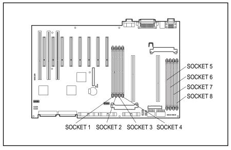
Figure 2-27. SDRAM DIMM socket locations
